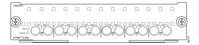
After you connect the cables to a configured port on the line card, it takes up to 35 seconds to initialize the line card and light the green LNK LED.
